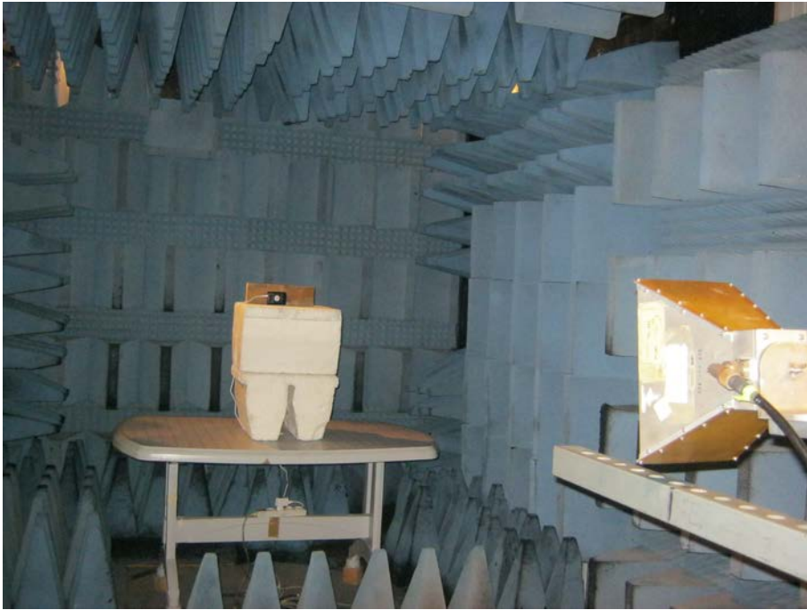
Figure 2. Intermodulated Radiated Emission Test
